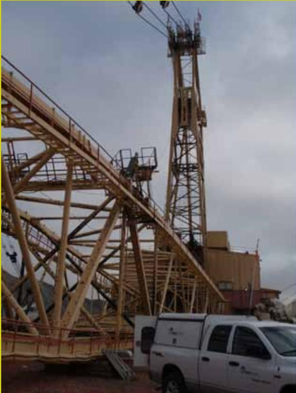
While increasing the bucket size is a popular way to increase production, it usually comes at the cost of an increase in the risk of catastrophic failure, increased maintenance and unplanned downtime. Repair welding on the aging major structural components has become commonplace during maintenance outages, and "Preventative Maintenance" has been replaced by a game of "chasing the cracks".
